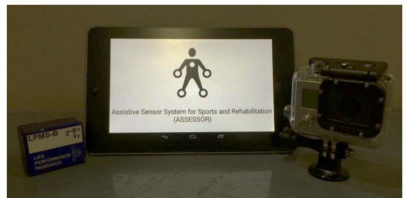
Fig. 3. Version 2 system: IMU, ASSESSOR, and high-FPS camera
