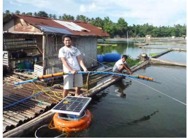
Fig. 3. One of the authors holding the sensor package before being attached to the floating field server. The two packages at 0.5 m and 2.5 m house DO, conductivity, and temperature sensors. Inside the buoy are the aerator pump, LED, Android phone, Arduino interface, battery and charge-controller.
