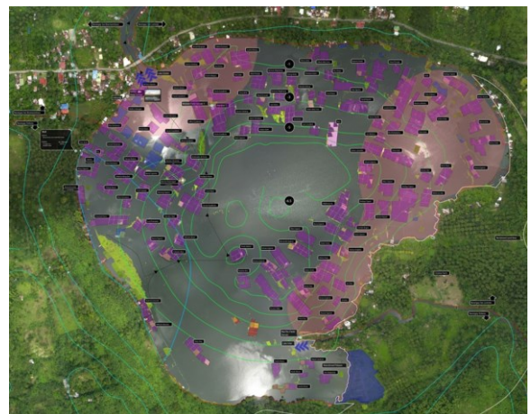
Fig. 10. Aerial image of Lake Palakpakin taken March 2013. This generated aerial map has been overlaid with bathymetry data and annotated information on fish pens. Based on image analysis, the fish pen coverage is at 13.86%, slightly higher than the legislated fish pen capacity of 10%.
