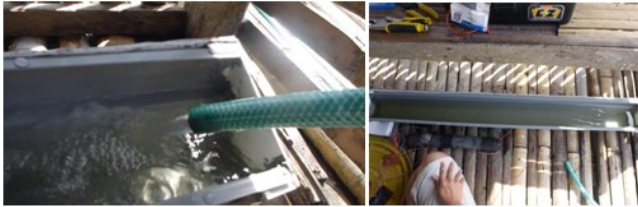
Fig. 5. Demonstration of pumping method in Lake Palakpakin. This method is used for the demonstration of our sensor measuring water turbidity at different depths. At right is the presence of sediments in water pumped from 3 m.
